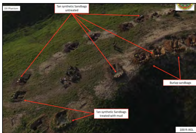
Synthetic sandbags shine "like light bulbs." From 100 ft AGL.
