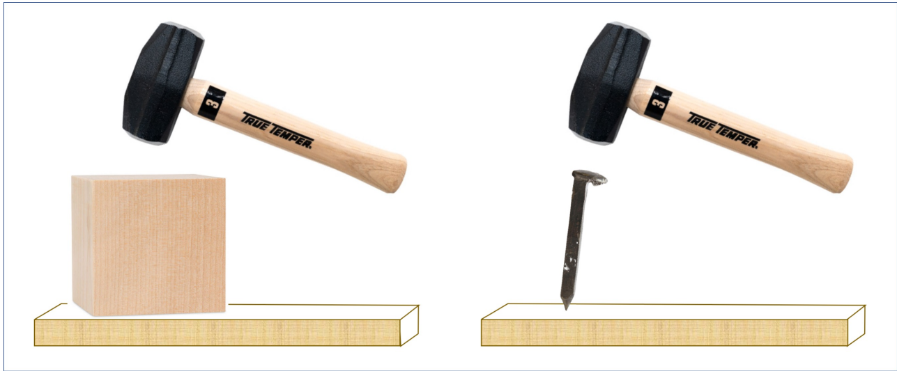
Figure 4. Main effort. The force of the hammer, dispersed, versus the same force, concentrated at a single point.
